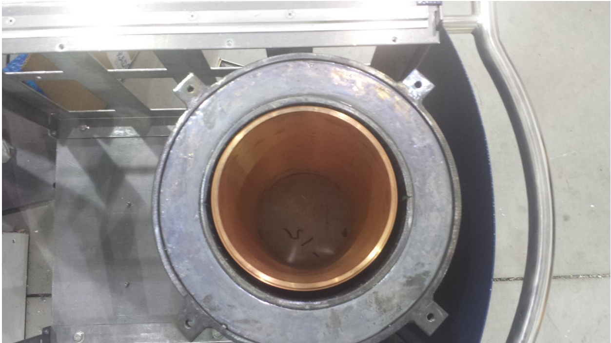
Picture 1. Lead shield with Copper lining to collect internal LaBr 3 (Ce) background.
