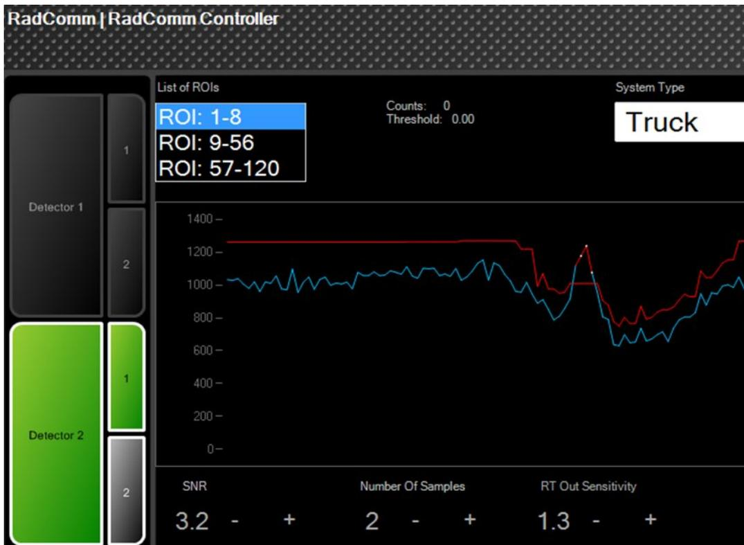
Fig 3. The background updating and alarm response of the PVT-based systems (time radiation profile)
